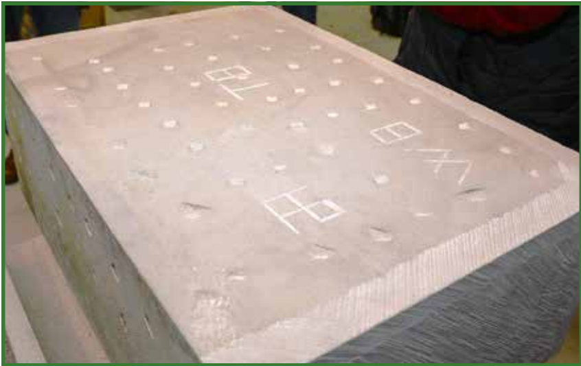
Figure 8 – Coursed stone displaying chisel carving
